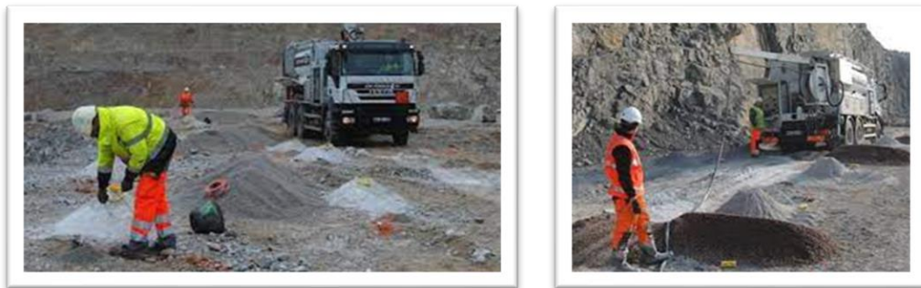
A quarry mining operation using a MEMU (source: EPC France website)
